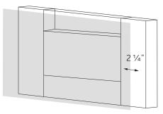
2. Secure the valve to the prepared wood blocking using the provided hardware. Ensure that the "cold" inlet is pointing to the right, and the "hot" inlet is pointing to the left. Use a level to ensure that the valve is straight and level.
