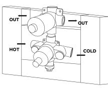
3. Route, assemble, and connect all in-wall piping as desired to and from the shower valve. Make all connections appropriately depending upon the type of pipe that is being used. For copper pipe, soldering will be required and should be completed by a licensed plumber. Apply plumber's tape to any threaded connections if applicable. Install any wood blocking that is necessary to support the piping and valve.
