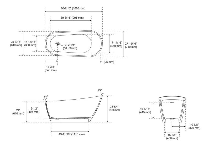
Dimensions of fixtures are nominal and may vary within the range of tolerance established by CSA B45.5-17/IAPMO Z124-2017.
