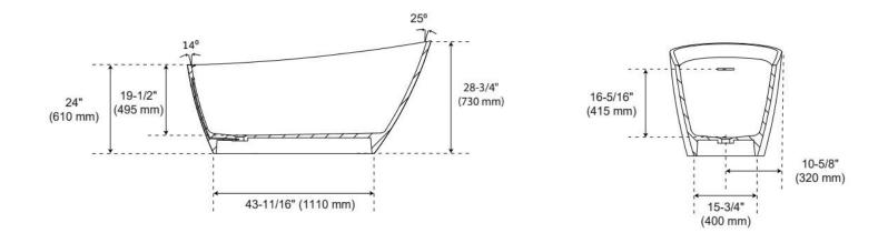
Dimensions of fixtures are nominal and may vary within the range of tolerance established by CSA B45.5-17/IAPMO Z124-2017.
