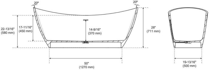
Dimensions of fixtures are nominal and may vary within the range of tolerance established by CSA B45.5-17/IAPMO Z124-2017.
