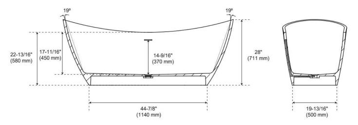
Dimensions of fixtures are nominal and may vary within the range of tolerance established by CSA B45.5-17/IAPMO Z124-2017.
