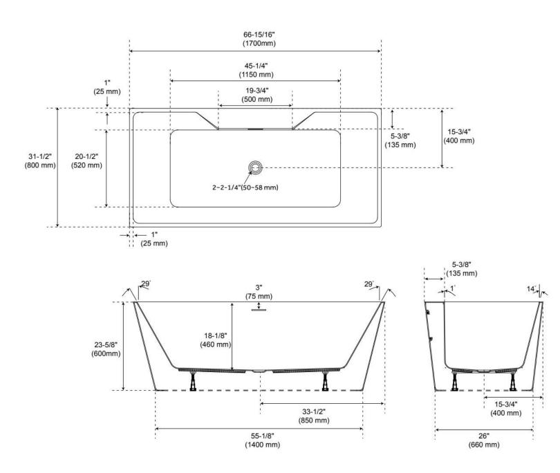
Dimensions of fixtures are nominal and may vary within the range of tolerance established by CSA B45.5-17/IAPMO Z124-2017.
