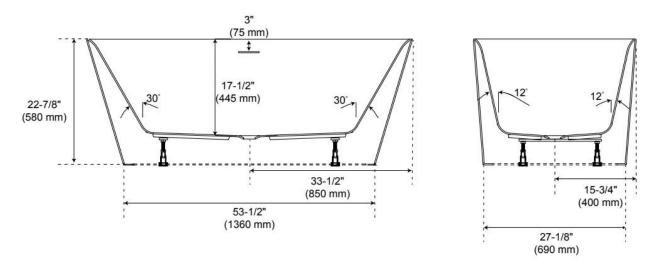
Dimensions of fixtures are nominal and may vary within the range of tolerance established by CSA B45.5-17/IAPMO Z124-2017.
