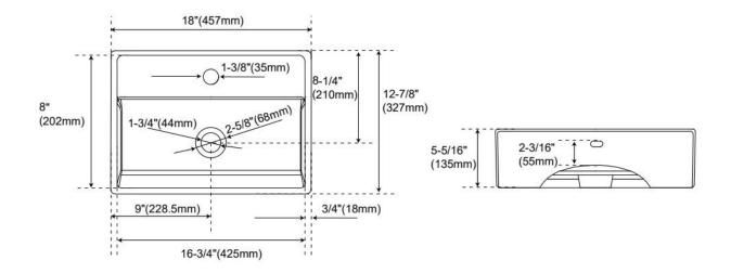
Dimensions of fixtures are nominal and may vary within the range of tolerance established by ASME A112.19.2
