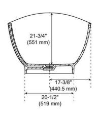
Dimensions of fixtures are nominal and may vary within the range of tolerance established by CSA B45.5-17/IAPMO Z124-2017.
