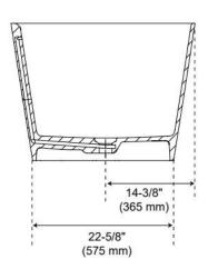
Dimensions of fixtures are nominal and may vary within the range of tolerance established by CSA B45.5-17/IAPMO Z124-2017.
