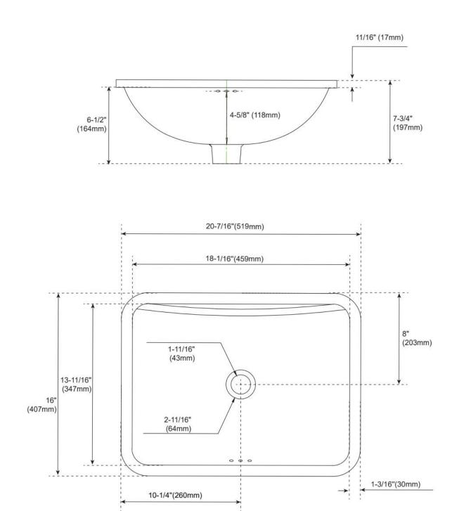
Dimensions of fixtures are nominal and may vary within the range of tolerance established by ASME A112.19.2.
