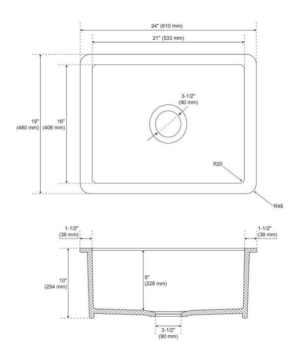
Dimensions of fixtures are nominal and may vary within the range of tolerance established by ASME A112.19.2.
