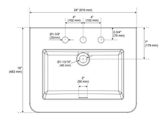
Dimensions of fixtures are nominal and may vary within the range of tolerance established by ASME A112.19.2
