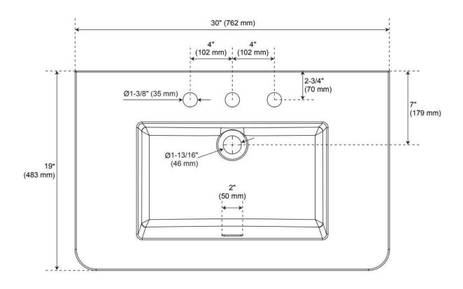
Dimensions of fixtures are nominal and may vary within the range of tolerance established by ASME A112.19.2
