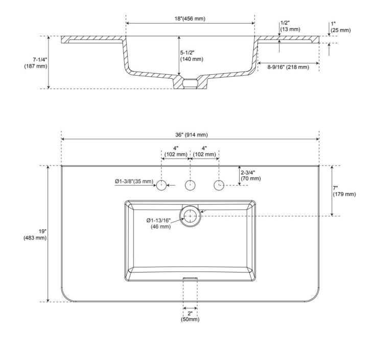
Dimensions of fixtures are nominal and may vary within the range of tolerance established by ASME A112.19.2
