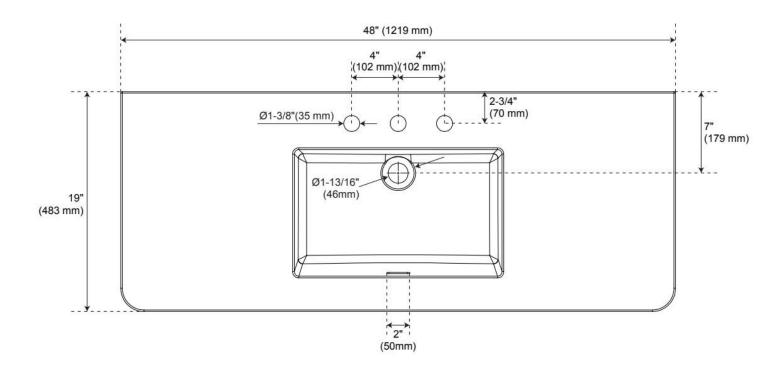
Dimensions of fixtures are nominal and may vary within the range of tolerance established by ASME A112.19.2
