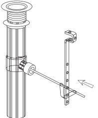
8. Attach the lift rod to the top of the link and secure it by tightening the thumb screw.
