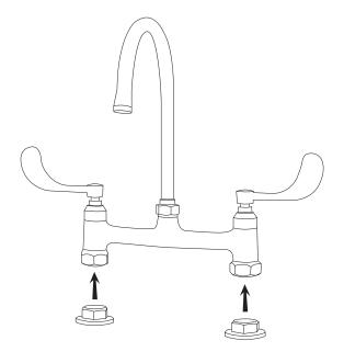
3. From below, slide the metal washers onto the threaded shanks. Thread the locknuts onto the shanks until hand-tight, then finish tightening using an adjustable wrench.
