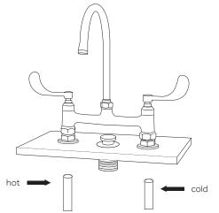
6. Once installation is complete, turn the main water supply back on from underneath your sink. Check for any leaks underneath.
