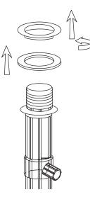
2. Set the flat rubber gasket over the drain hole in your sink, then insert the flange into the drain hole.
