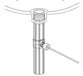
6. If not already installed, insert the faucet's lift rod into its designated hole on the back of the faucet.
