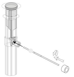
5. Position the drain so that the lever is facing the back of the fixture, in line with the faucet's lift rod. While holding in place, hand tighten the lock nut until secure then finish tightening with a basin wrench. Be careful not to overtighten, which can crack a fragile sink.
