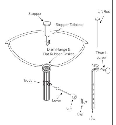
1. Remove the flange by unthreading it from the drain body. Remove the flat rubber gasket as well.
