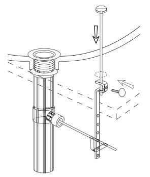
9. Make any final adjustments to the positioning of the link and drain lever as needed. Adjust until the drain fully opens and closes.
