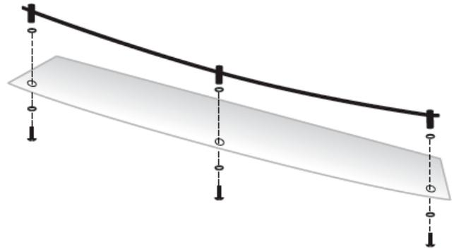
4. To mark the escutcheon placement, find the center point of the line that you drew on the wall. Make two marks to the right and left of the center, at an equal distance. The escutcheons should be 1-2" in from the outer edges of the glass shelf.
