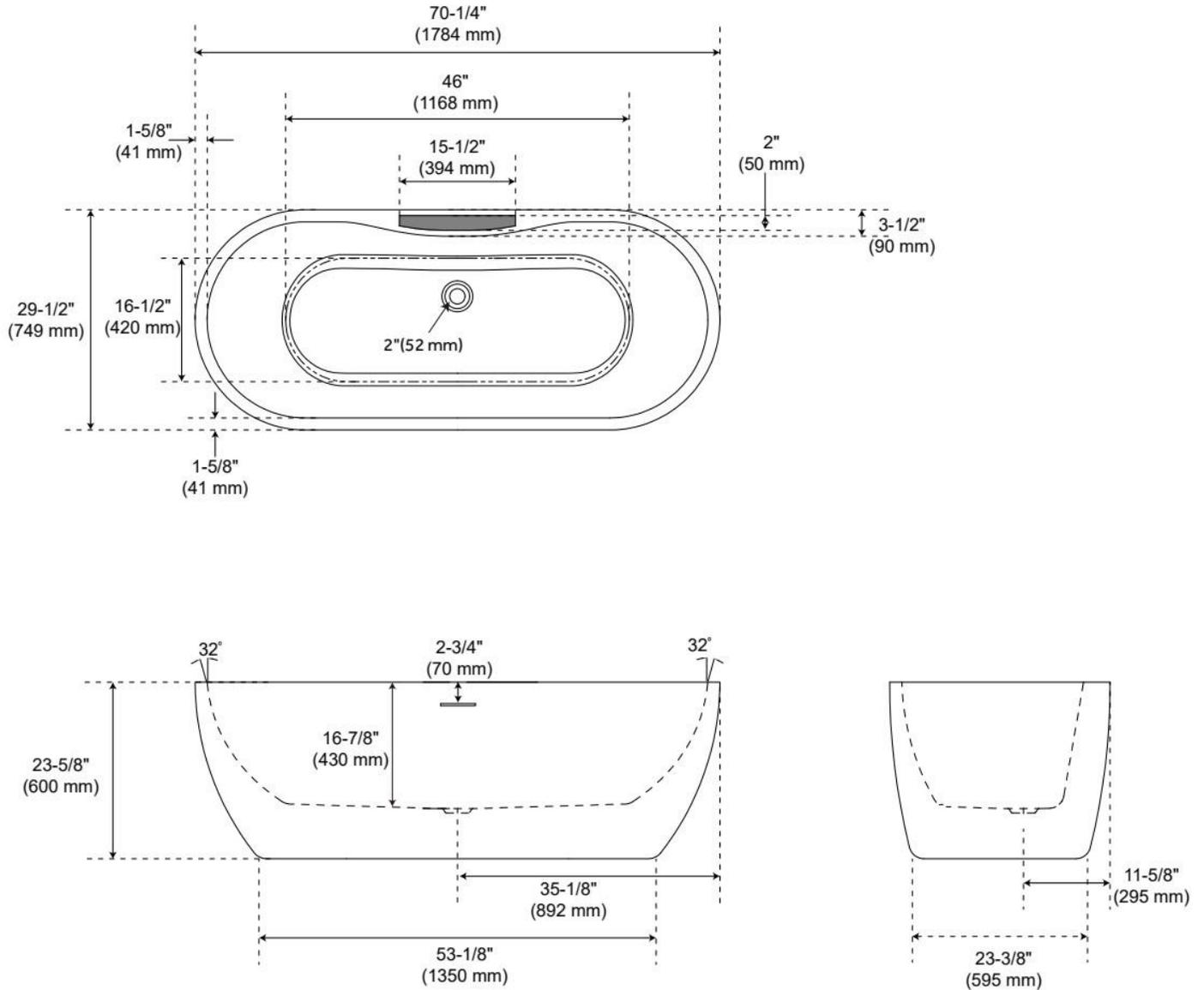
Dimensions of fixtures are nominal and may vary within the range of tolerance established by CSA B45.5-17/IAPMO Z124-2017.
