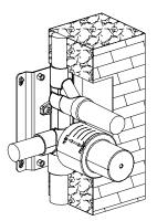
2. Put the protective covers on the valve body and finish the shower wall.
