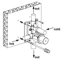
1. Install the valve body. Wrap the threaded portion of the joints in Teflon tape and connect the water inlet and outlet.
