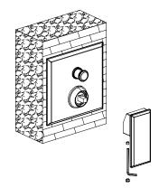
4. Install the escutcheon, and handle. Tighten the set screw with an Allen wrench to secure.
