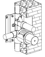
2. Put the protective covers on the valve body and finish the shower wall.
