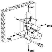
1. Install the valve body. Wrap the threaded portion of the joints in Teflon tape and connect the water inlet and outlet.
