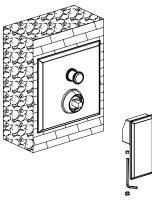
4. Install the escutcheon, and handle. Tighten the set screw with an Allen wrench to secure.
