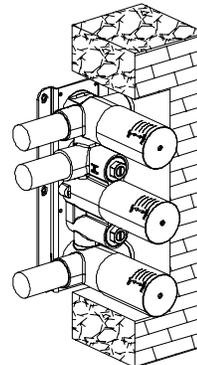
1. Install the valve body. Wrap the threaded portion of the joints in Teflon tape and connect the water inlet and outlet.
