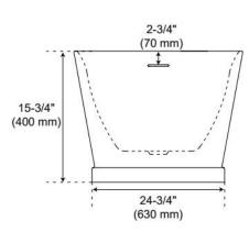
Dimensions of fixtures are nominal and may vary within the range of tolerance established by CSA B45.5-17/IAPMO Z124-2017.
