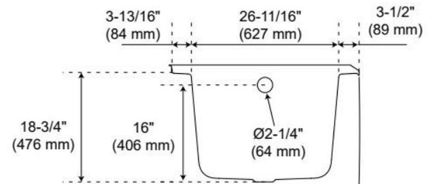
Dimensions of fixtures are nominal and may vary within the range of tolerance established by CSA B45.5-17/IAPMO Z124-2017.
