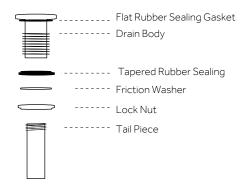
2. Place thread sealant on the threaded section of the tail piece and reattach to the drain body.
