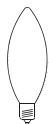
Light Bulb (E12 60 watt maximum) Ampoule (E12 60 watts maximum) Bombilla (E12 60 vatios máximo)
