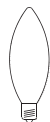
Light Bulb (E12 60 watt maximum) Ampoule (E12 60 watts maximum) Bombilla (E12 60 vatios máximo)
