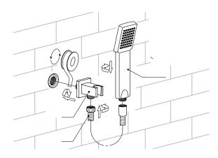
50. When installation is complete turn the faucet on, check to make sure that the hot and cold supplies are working correctly. Diver the water to each shower head output and hand shower and allow the water to flow for approximately 60 seconds.
