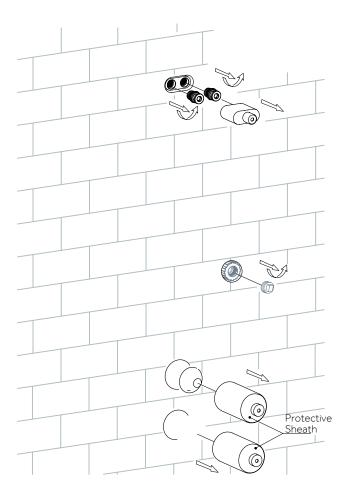
24. For masonry wall installation, wrap plumbers tape around the threaded connections and attach to the valve body.
