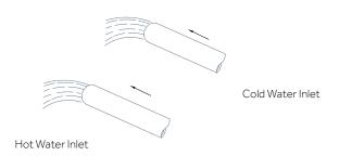
15. Connect the inlet pipes. Wrap plumblers tape around the threaded portion of the plug. Insert the plug into the 90° female elbow.
