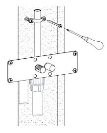
42. Place the protective sheaths over the pipe inlets and install the finished wall material.
