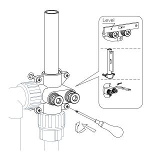
10. Mark the location of the mounting holes on the valve body in the installation location. Use a level to ensure the holder is alighned properly.
