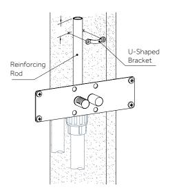
40. Drill mounting holes and insert wall anchors.
