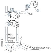
38. Remove the protective sheath and run water to test the pressure and ensure there are no leaks.
