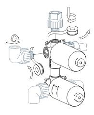
25. Wrap plumbers tape around the threaded connections and attach to the shower holder.
