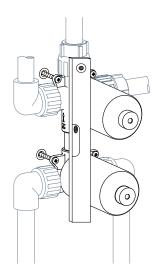
$14.\, \text{Turn}$  the water on to flow water through the pipes to clear out any dirt and debris.
