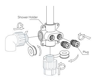
4. Determine the locations of the valve body and shower head. Connect the inlet pipe to the inlet joint. Install the 90° female elbow in thehand-shower holder location.
