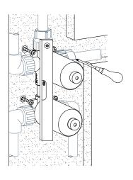
36. Turn the water on to flow water through the pipes clear out any dirt and debris.
