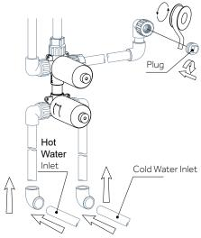
16. Remove the protective sheath and run water to test the pressure and ensure there are no leaks.
