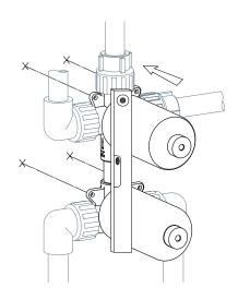
11. Drill mounting holes with the appropriate drill bit and insert the wall anchors.
