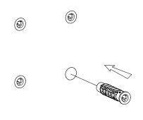
8. Loosely attach the shower holder to the wall with self-tapping screws.
