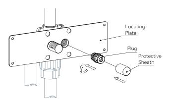
28. Mark the location of the mounting holes on the locating plate in the installation location. Use a level to ensure the holder is aligned properly.
