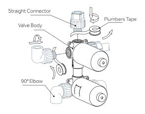
3. Wrap plumbers tape around the threaded portion of the plugs and attach to the shower holder.
