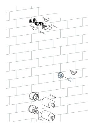
44. Turn the water on to flow water through the pipes to clear out any dirt and debris.
