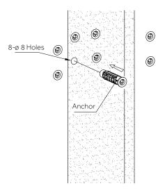
30. Loosely attach the plate to the wall with self-tapping screws.
