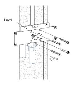
$32.\,\mbox{Mark}$  the location of the mounting holes on the valve body.
