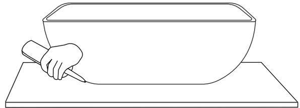
4. Remove any excess sealant with a damp cloth to complete installation.
