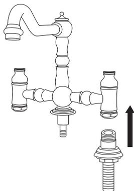
3. Remove the brass lock nuts from the threaded shanks and insert the faucet into its designated mounting holes on the mounting surface.
