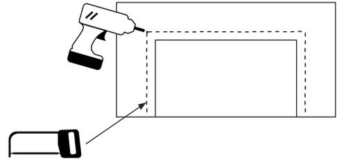
3. Determine placement of clip brackets as indicated by template. Pre-drill holes according to the method recommended for your countertop material.
