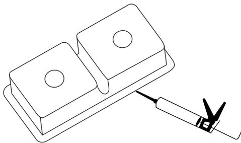
5. Insert clips into the channel "3 clips placed in the front and back and two on each side". Arrange the clips evenly around the sink. The clips should be parallel to the channel.
