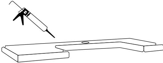
6. Position and align sink over opening. Press the sink onto the sealant seal.
