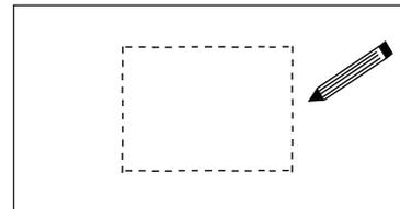
3. Drill a pilot hole inside the cutout line. Then proceed to cut out the countertop opening by carefully following the line traced on the countertop.
