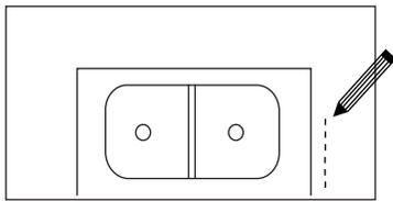
2. Drill a pilot hole inside the cutout line. Then proceed to cut out the countertop opening by carefully following the line traced from the template.
