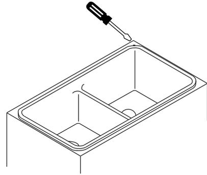
8. Wipe off any excess silicone sealant with a damp cloth. Apply additional sealant if necessary.
