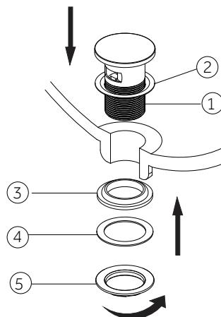
8. Slide the nut (2) over the tail pipe (3). Place the washer (1) into the nut and tighten. Do not over tighten.
