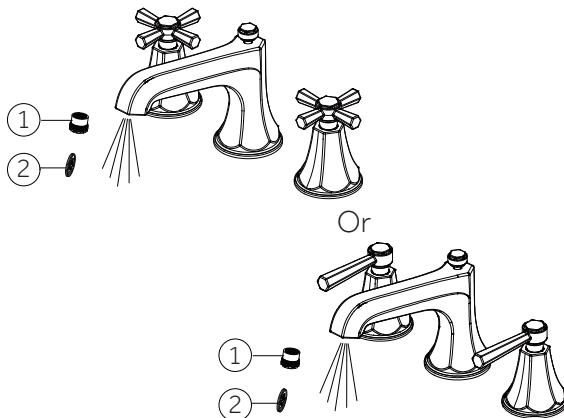
10. If faucet leaks from spout, shut off the water supplies and replace the cartridge (1).
