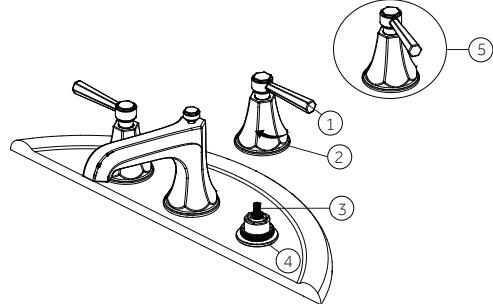
4. Align tabs (1) and (2) on quick connects (3). Push quick connect housing firmly upward and snap onto receiving tube tab. Pull down moderately to ensure connection has been made. If it is necessary to remove quick connect, squeeze tabs on hose between index finger and thumb, then pull down to disconnect.
