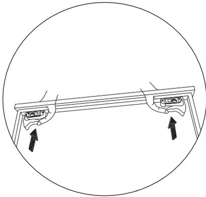
2. Remove the screw from the shelf supports if needed. Lift up the shelf and reposition the shelf supports to the desired height. Rest the shelf on the shelf supports and reinstall screws (if desired).
