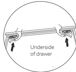
3. Re-install the drawers by pulling the inner slides fully to the front. Sit the drawer on top of the inner slides while inserting the hooks at the back of drawer. Push drawer so that the glides and trigger will engage.
