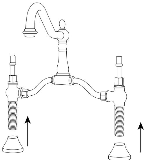
3. From beneath the sink, slide the rubber washers onto the faucet body. Thread the locknuts onto the threaded shanks until hand tight. Tighten firmly.
