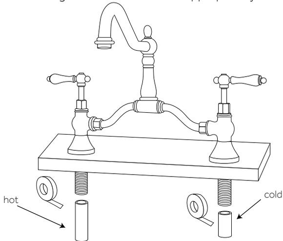
6. Once installation is complete, turn the main water supply back on from underneath your sink. Check for any leaks underneath.
