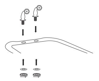
3A. Attach the faucet body to the installed deck couplers. Apply thread sealant or plumber's tape to the threads before tightening. Tighten firmly using an adjustable wrench, then finish tightening the lock nuts, securing the faucet to the deck.
