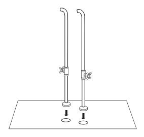
2B. Apply plumber's tape or thread sealant to the threaded outlets on the back of the faucet body. Attach the faucet to the installed supply lines. Tighten firmly using an adjustable wrench.
