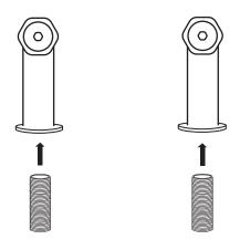
2A. Insert each of the deck couplers into their prepared mounting holes. From underneath, slide the metal washer onto each threaded shank, followed by the lock nut. Thread the lock nut onto the shank until hand-tight. Do not fully tighten yet.
