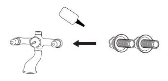
2C. Insert the faucet into its prepared mounting holes. From behind, thread the lock nuts onto the threaded shanks to secure the faucet to the tub.
