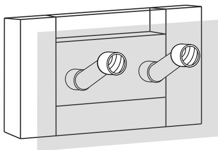
2D. Apply plumber's tape or thread sealant to the exposed threads of the pipe nipples installed in the wall. Attach the provided wall mount couplers to the pipe nipple. Tighten firmly using an adjustable wrench.
