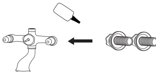
2C. Insert the faucet into its prepared mounting holes. From behind, thread the lock nuts onto the threaded shanks to secure the faucet to the tub.
