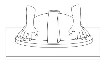
7. Carefully turn the countertop and sinks over. If needed, reposition the sinks by slightly loosening the wing bolts and adjusting.
