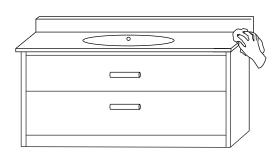
3. If you are installing a side-splash and/or back-splash, place a generous amount of silicone sealant on the back of it and press it into place against your bathroom wall. Fill any gaps that are left with silicone sealant. Wipe away any excess sealant with a damp cloth.
