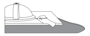
4. Remove the sink from the countertop. Apply a bead of silicone sealant around the top edge of the sink rim.
