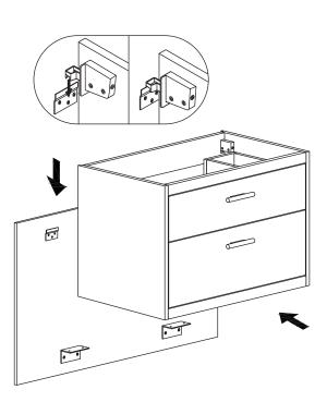
4. Adjust the mounting attachment as required. Lower screw adjusts vertical position. Upper screw adjusts depth.
