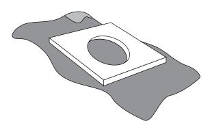
2. Position the sink over its cutout on the countertop. Make sure the sink is centered with the faucet hole and is evenly spaced between the bolt holes.
