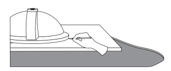
4. Remove the sink from the countertop. Apply a bead of silicone sealant around the top edge of the sink rim.
