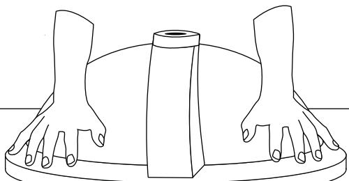
6. If sink clips were included, at each of the bolt holes in the countertop, attach the sink clips by placing the long end of the bracket flat against the sink lip. Screw the wing bolts through the brackets and bolt holes and tighten.
