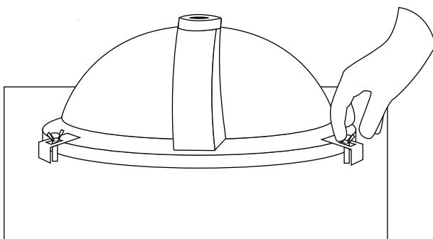
7. Carefully turn the countertop sink over. If needed, reposition the sink by slightly loosening the wing bolts and adjusting.
