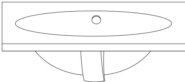
8. Wipe away any excess sealant with a damp cloth, and proceed to installing the countertop. Allow all silicone to dry for 24 hours.
