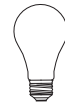
Light Bulb (A19 100 watt maximum) Bombilla (A19 100 vatios máximo) Ampoule (A19 100 watts maximum)
