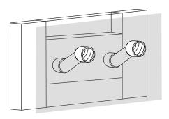
2C. Apply plumber's tape or thread sealant to the exposed threads of the pipe nipples installed in the wall. Attach the provided wall mount couplers to the pipe nipple. Tighten firmly using an adjustable wrench.
