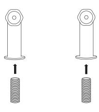
2A. Insert each of the deck couplers into their prepared mounting holes. From underneath, slide the metal washer onto each threaded shank, followed by the lock nut. Thread the lock nut onto the shank until hand-tight. Do not fully tighten yet.
