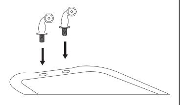
3A. Attach the faucet body to the installed deck couplers. Apply thread sealant or plumber's tape to the threads before tightening. Tighten firmly using an adjustable wrench, then finish tightening the lock nuts, securing the faucet to the deck.
