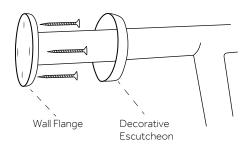
6. Attach the grab bar to the floor with the mounting screws provided. Slide or thread the decorative escutcheon over the floor flange and press firmly in place to complete installation.
