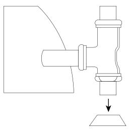
14. When your tub is in place and all connections have been made, fill the tub with water to check for any leaks from the connections. Verify that the drain and overflow is working properly.
