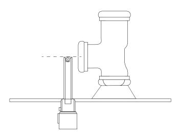
3. Carefully set the tub back into position and adjust the leveling feet as necessary. If your tub does not have leveling feet, shims may be used. Once level, apply a generous bead of silicone on the bottom of the feet. This will prevent the tub from shifting after installation.
