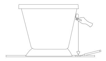
2. Move the tub away from the installation location so that the floor plumbing can be installed. Place the drain pipe at the appropriate height for the waste and overflow piping. To determine this, you will need to temporarily fit your drain pipe into the tub and measure from the floor to the center of the drain pipe.
