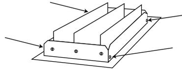
2. Using the removed screws, attach the spring clips to the register as shown.
