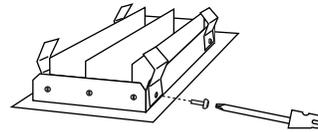
**Note:** The mounting points for spring clips may be on the long or short side of your register depending on the style of register.
