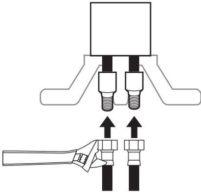
6. Briefly turn on the main water supply to ensure that there are no leaks. Once you have determined that there are no leaks, turn the water supply back off and continue with the installation.
