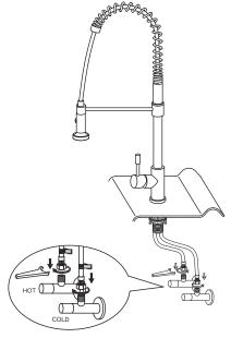
6. Once installation is complete, turn the main water supply back on from underneath your sink. Check for any leaks underneath.
