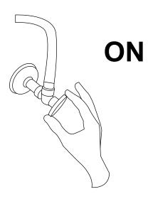
7. Remove the sprayer from the spout. Turn the faucet on and allow the water to flow for approximately 60 seconds. Ensure that there are no leaks, and that both hot and cold water are running properly. Reattach the sprayer.
