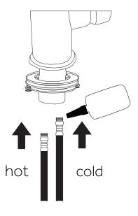
3. Remove the lock nut, metal washer, and rubber gasket from the faucet body. Insert the faucet body through the mounting hole in your counter top. Position the faucet so that the handle is on the left, as shown.
