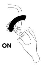
7. Remove the hand sprayer by unthreading it from the sprayer hose. Turn the faucet on for approximately 60 second to remove any dust or loose sediment from the water lines, and to ensure that there are no leaks. Check to ensure that both hot and cold water are running properly. Reattach the sprayer and turn it on. Allow the sprayer to run for another 60 seconds, and check for any leaks.
