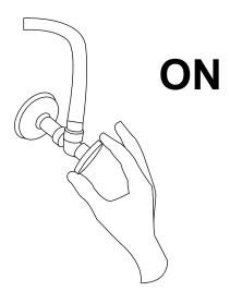
6. Remove the aerator from the spout. Turn the faucet on and allow the water to flow for approximately 60 seconds. Ensure that there are no leaks, and that both hot and cold water are running properly. Divert water to the sprayer setting and allow it to flow for another 60 seconds.
