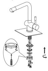
4. Apply plumber's tape or thread sealant to the threading on each of the faucet's water lines, and connect the main water hoses to the faucet. Ensure that you are connecting the hot and cold lines appropriately.
