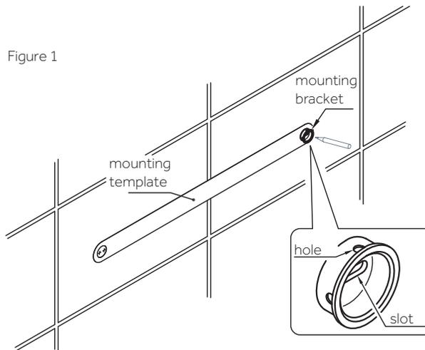
1. Position the mounting template on the wall at the desired installation location (Figure 1). Hold the mounting brackets in their location at each end of the template, and mark the location of the mounting holes. Make two marks in each slot, as each mounting bracket will require two screws. Ensure that the mounting template is level before making marks.
