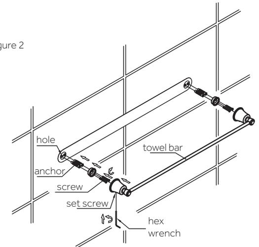
3. Insert anchors into the drilled holes. Fasten the mounting brackets to the wall, as shown, using the provided screws (Figure 2).
