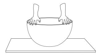
3. If desired, apply a continuous bead of silicone sealant around the perimeter of the sink base for additional stability.
