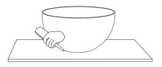
4. Remove any excess sealant with a damp cloth to complete installation.
